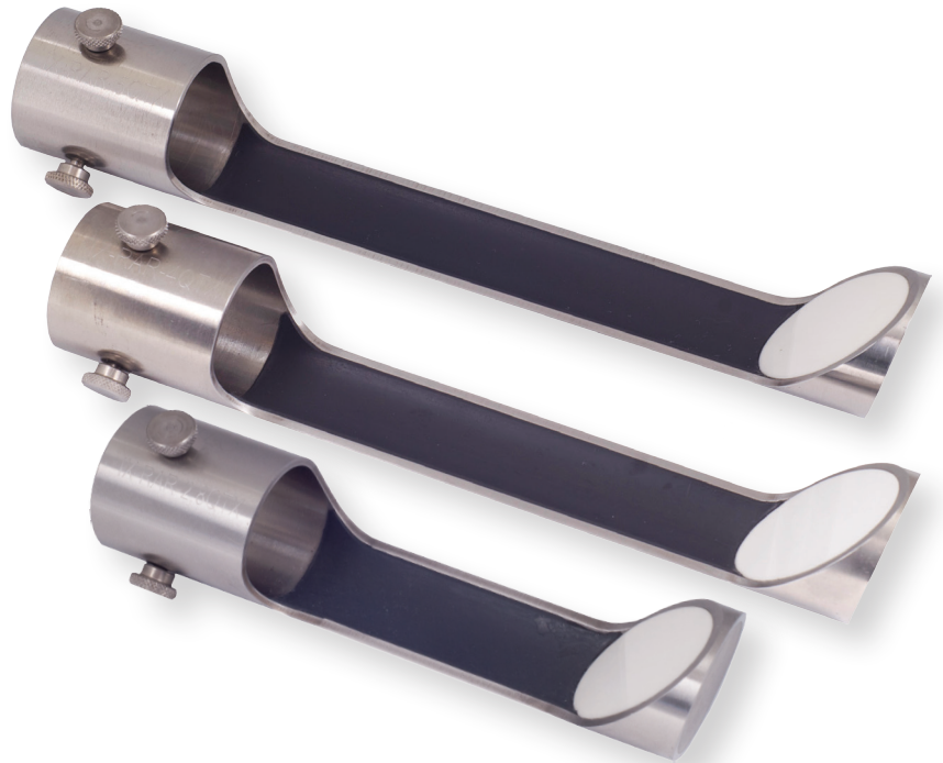
Right angle mirror for IX (1" Nom. OD) standard housing with variable water path from end of transducer to center of 45 degree mirror.
