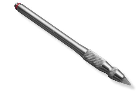
This high frequency, focused delay line transducer, is used for thickness gauging from .007" to .3" in steel. It is ideally suited for curved/irregular surface testing. Includes .0625" or .125" contact tip.
