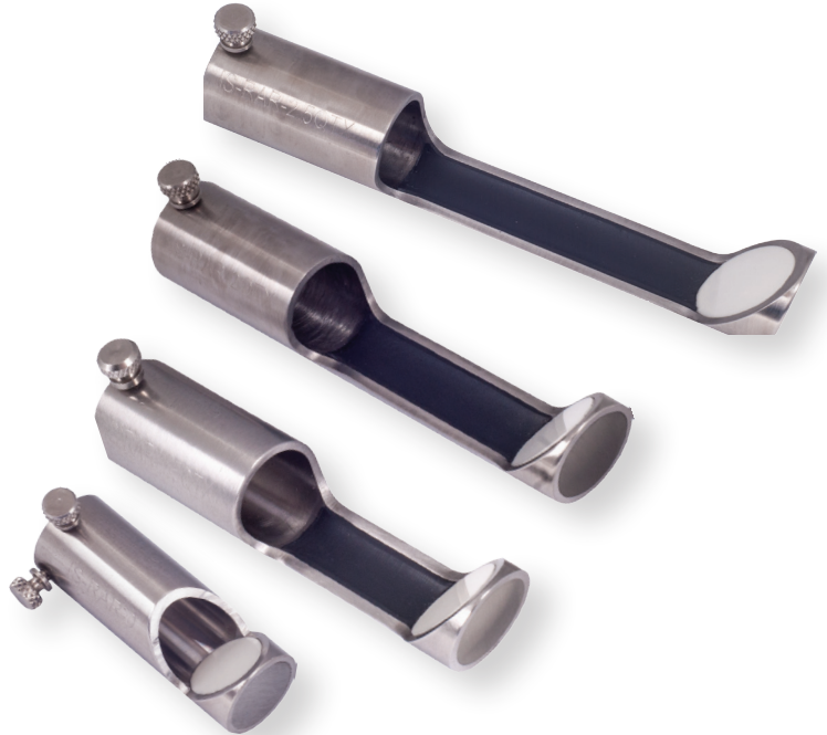
Right angle mirror for IS standard housing (0.625 Nom. OD) with variable water path from end of transducer to edge of 45 degree mirror.
